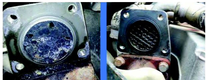
EGR Coolers before and after
