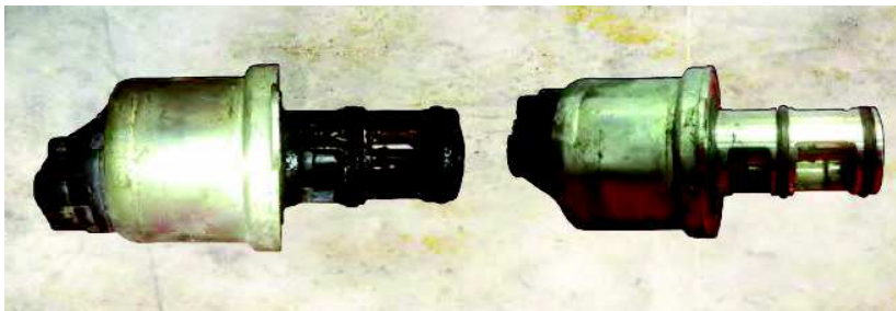
EGR Valves before and after cleaning
