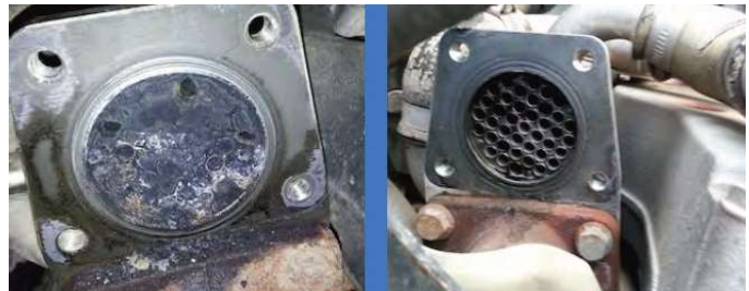
EGR coolers before and after
