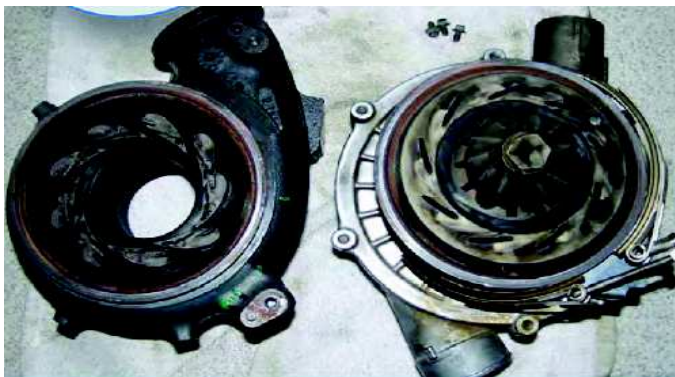
Turbo charger before and after
