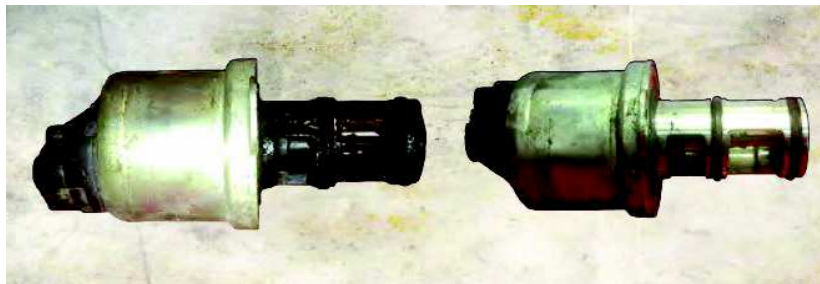
EGR Valves before and after cleaning
