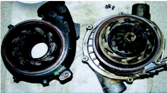
Turbo charger before and after
