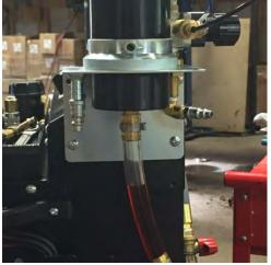
Step 2. On the right hand side of machine, remove the top 90 degree elbow from the machine.
