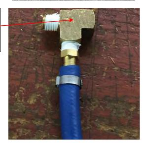
Step 4. Attach the hose from the fluid injector to the top hose barb, and secure with clamp.
