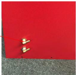
Step3. Take the adapter from the blue hose and put 90 degree fitting into this adapter. - Then screw the adapter into were you took the 90 degree adapter out of the machine.
