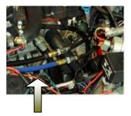
Disconnect the return line which returns the fuel back to the fuel tank
