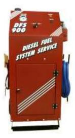
A cleaning fluid is circulated through the fuel system, while the vehicle is running. This process isolates the injector pump, lines and injectors, allowing the cleaning fuel to remove varnish, gum, carbon and other contaminants from the complete fuel system and combustion chamber.
