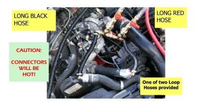
Remove the top radiator hose at either the engine block or at the radiator whichever is the most accessible. If desired pour a radiator flush chemical into the radiator hose or into the radiator.
